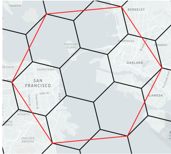
Figure 2.10: Hierarchical indexing structure of the H3 system (Source: Uber Engineering [Eng]).
